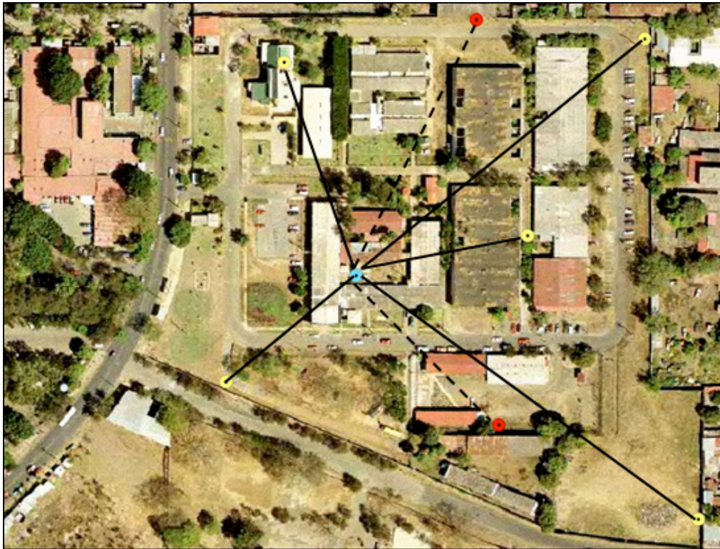
Figure 4. Configuration of the small seismic array at INETER, Managua (4.5 Hz sensors)
